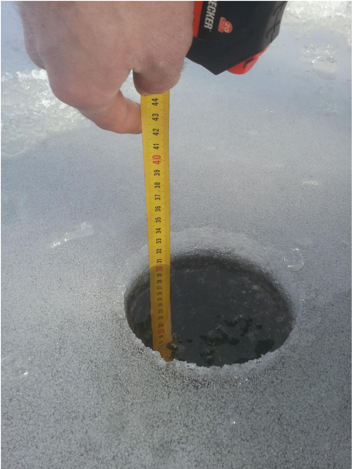
Pic 1. Ice thickness at point 1
